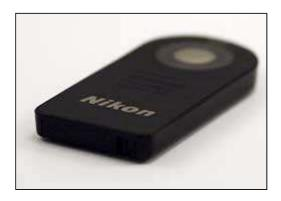
The remote uses infrared (IR), just like your TV remote control uses. In fact if you have a re-programmable TV remote there's a good chance you can program it to trigger your camera as well. Set the D70 into remote mode and while in front of the camera go through various programming defaults on the remote. I think Sanyo or Samsung TVs often work.
