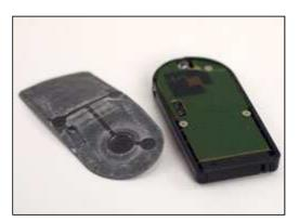
On the other side of the circuit board are some electronic parts, including the translucent white IR LED at the tip. There's one integrated circuit, which takes care of generating all of the IR signals sent to the camera.
