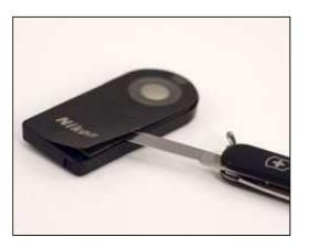
I peeled the bottom half up, found two small screws, removed them and then assumed that that was it and tried to pull it apart. Turns out there's a third screw at the top and the printed circuit board (PCB) breaks pretty easy. Don't do that. Peel the whole decal off, gently, and set it off to the side where it won't get dirty. If you break the circuit board like I did you'll have more soldering to do.
