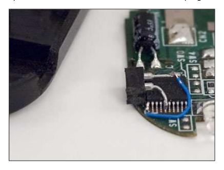
As you can see, pin #1 and pin #5 are used to trigger the remote. Double check for solder blobs and shorts when you are done. Here's a picture of the
