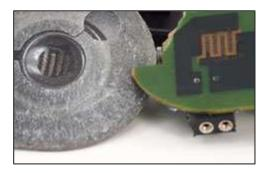
What we are going to do is hook up some wires to the chip in the same place that the button is hooked up. This lets us add an external button. There are two ways you can do this. If you are really talented at soldering or have a buddy who is and have some very thin wire you could attach the wire on the top and route the wire out the side. Those dark areas on the board and the two through holes are where you'd connect.
